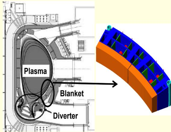
A Schema of Heat Transfer from PFM (500°C) to Coolant (300°C)
