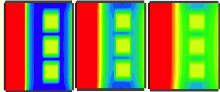
*Temp. Gradient Exists between PFM and Coolant*
