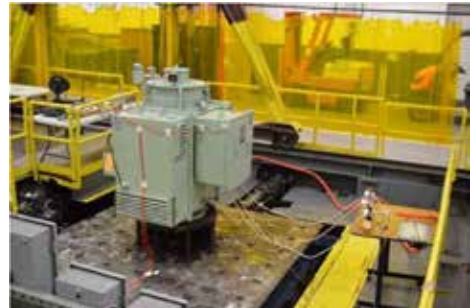
Hyosung 150 HP Vertical Motor - Seismic Test Setup
