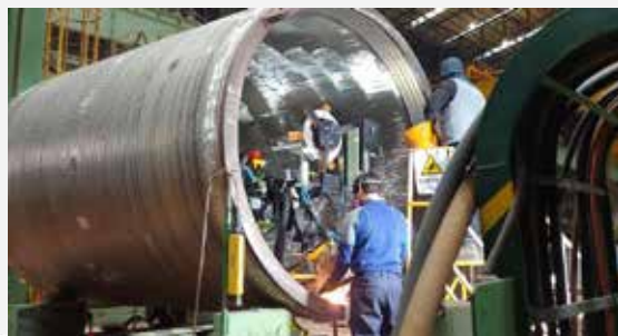
Cladding Distortion Trial (ESW)
