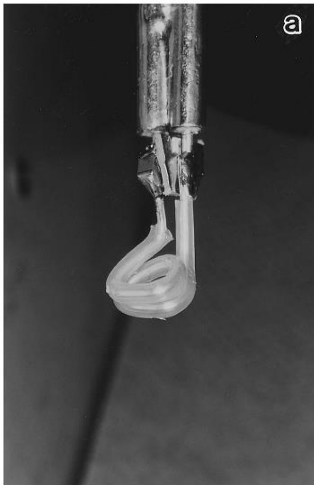
Fig. 3. The specially designed resonator for use in the mouth of living rats. (a) Illustration of the twin spiral loop gap resonator which has 5.0 mm internal diameter; it is a varactor tuned surface coil. (b) Illustration of the measurement in live rats; the EPR signal is detected from the upper pair of incisors, under anesthesia.
