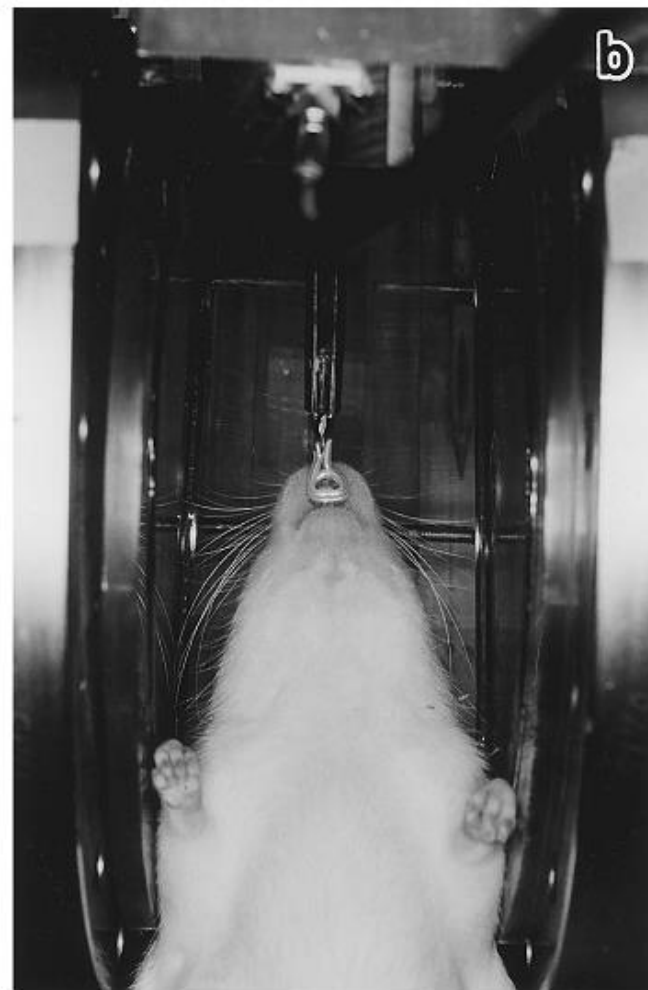
Fig. 3. The specially designed resonator for use in the mouth of living rats. (a) Illustration of the twin spiral loop gap resonator which has 5.0 mm internal diameter; it is a varactor tuned surface coil. (b) Illustration of the measurement in live rats; the EPR signal is detected from the upper pair of incisors, under anesthesia.
