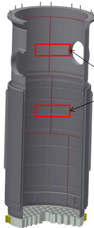
Fig. 4 Core barrel upper & lower girth weld
