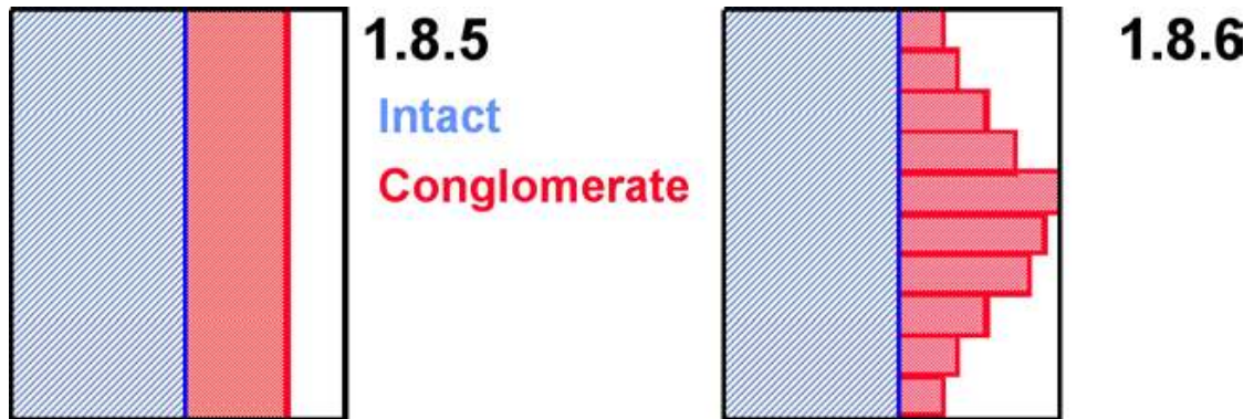
그림 A.3.1.1-4 Flow blockage for a cell, as predicted by the COR candling model (Comparison of MELCOR version 1.8.5 and 1.8.6)
