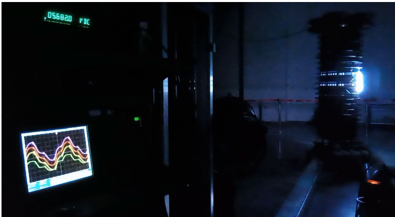
550 kV in-air test was successful
