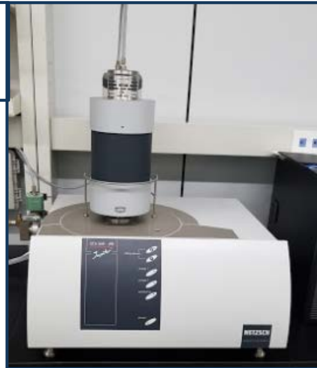
DSC-TGA Netzsch STA449F5
