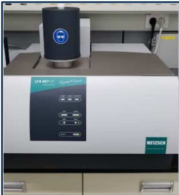
Laser Flash Analyzer Netzsch LFA467HT
