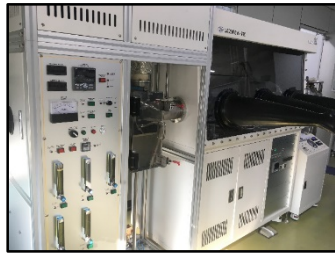
Glove Box - Tube furnace
