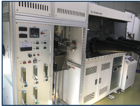
Glove Box - Tube furnace
