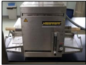
High T. Tube furnace
