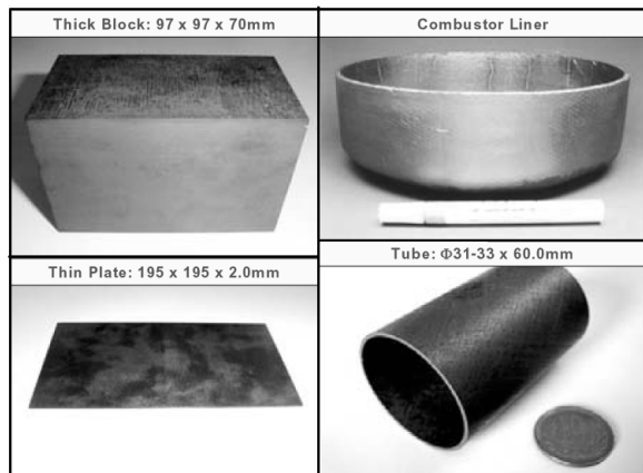
Fig. 11. Shape Flexibility of NITE SiC/SiC
