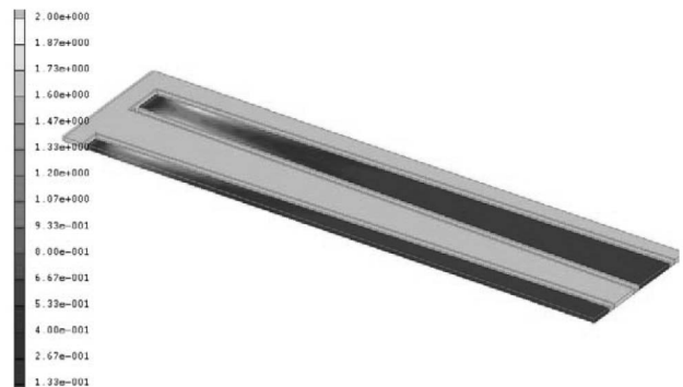
Fig. 17. Calculated Von Mises Stress Profile in the Breeding Unit (emphasizing stress distribution inside the breeder zone.)
