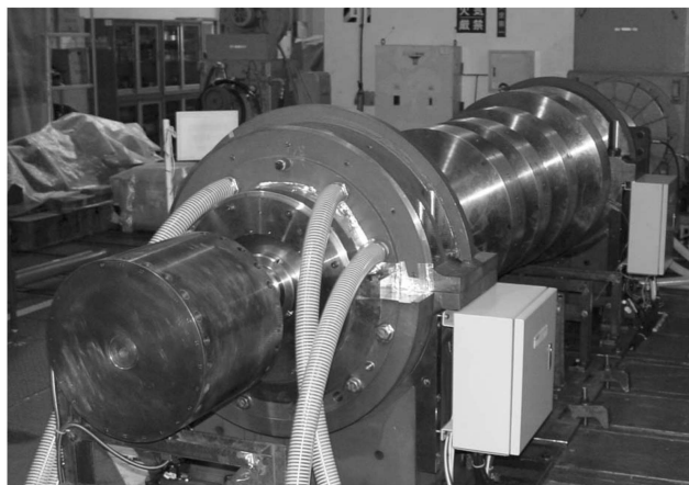
Fig. 3. Rotor of 1/3 Scale Magnetic Bearing Test
