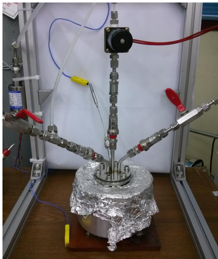
Fig. 4. The reactor covered by heater and measurement lines
