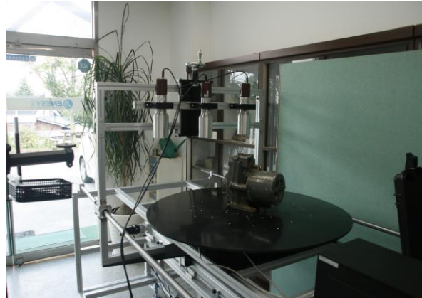
Fig. 4. Radioactive inventory evaluation system using 3D shape and multiple radiation measurement
