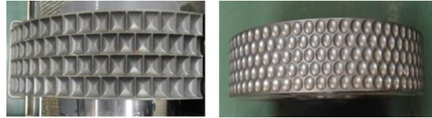
Fig. 1. The shape of the pellet pocket of the roll tyre
