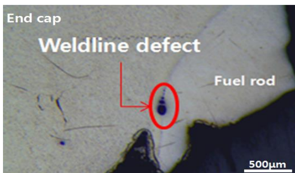
Figure 2. Weld line defect of the fusion line in the fuel rod weld zone
