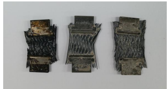
Fig. 2. Specimens of SiC-fiber fabric impregnated using a PCP-dissolved n -hexane and/or divinylbenzene solution.
