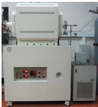
Figure 4. Apparatus (tube furnace) for high temperature oxidation of coated Zr alloys in steam
