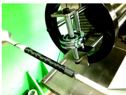
Fig. 1. Filament winding on SiC coated graphite rod.
