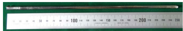
Fig. 1. U-10wt.%Zr-5wt.%Mn fuel slug, fabricated by innovative casting method under atmospheric atmosphere during whole casting process.
