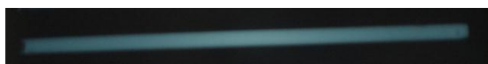
Fig. 3. A gamma radiography of U-10wt.%Zr fuel slugs fabricated by vacuum injection casting
