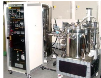
Fig. 1. An appearance of the vacuum injection casting apparatus.
