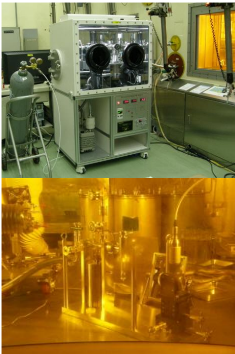
Fig. 1 Laser puncturing system in IMEF
