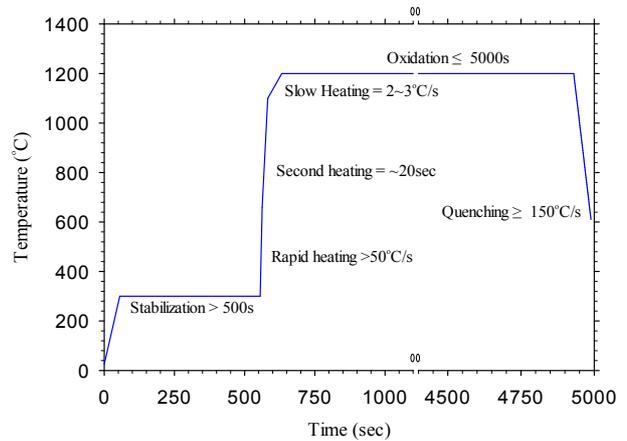
Fig 2. Temperature control to reduce the overshoot in sample temperature
