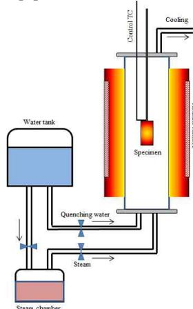
Fig 1. Schematic diagram of the LOCA simulation test equipment
