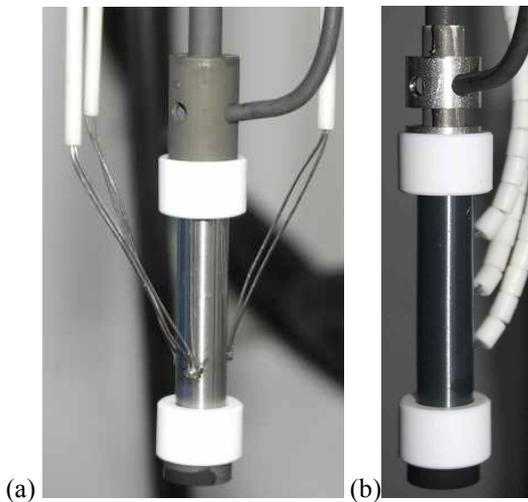
**Fig 4. TC welded sample tubes for (a) circumferential and (b) axial temperature variations measurement.**
