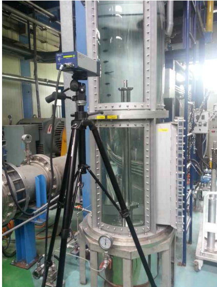
Fig. 2. The picture of the out-pile test for the vibration measurement of 12F-28K at the single channel test loop
