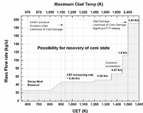
Fig. 3. Necessary flow rate for removal of core heat using CET
