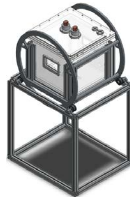
Fig. 2. 3D drawing of pool boiling apparatus
