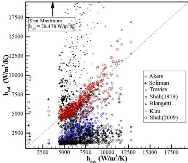
Fig. 1. The prediction of the correlations of condensation heat transfer coefficient with the experimental data of Khun(Laminar)
