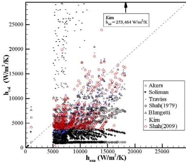
Fig. 2. The prediction of the correlations of condensation heat transfer coefficient with the experimental data of Khun(Turbulent)
