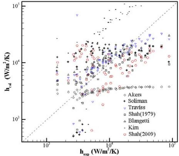
Fig. 3. The prediction of the correlations of condensation heat transfer coefficient with the experimental data of Lee
