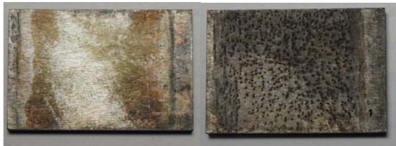
Fig. 3. The left photograph does not show any pits(FAC) (ASTM A336 F22V), and the right photograph shows more pits(SA 508 Gr.3)
