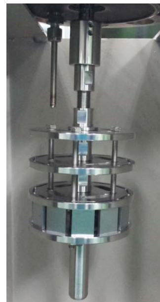
Fig. 3. Feature of the test specimen holder.
