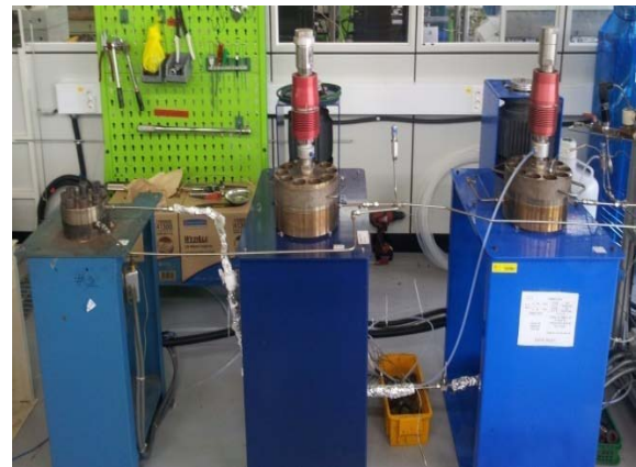
Fig. 2. Rotating cylinder combined in the autoclave
