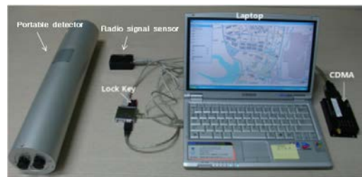
Fig. 1. Environmental radiation detection and analysis system
