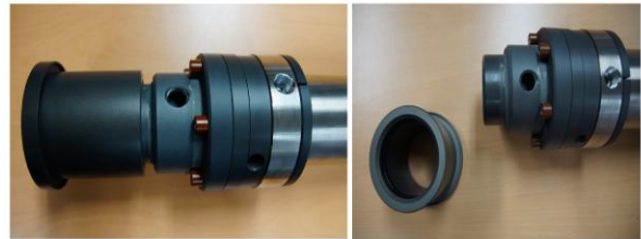
Fig. 3 Photos of target system for I-123
