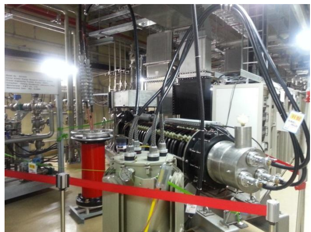
Fig. 3. Modulator and klystron system for 20MeV DTL
