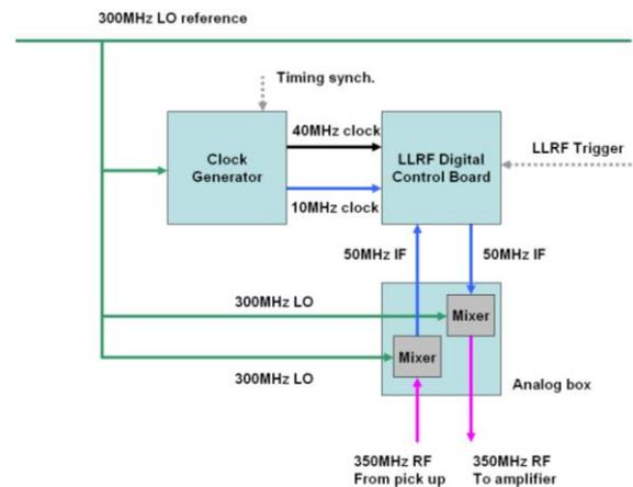
Fig. 1. Block diagram of the LLRF RF control system
