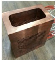
Heating Module (made of Copper)
