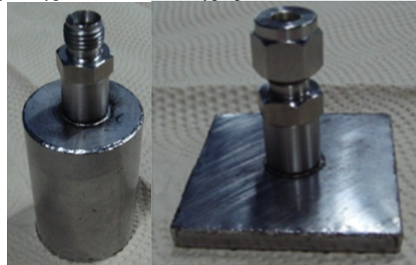
The annular capsule type permeation sensor (left) The plate type permeation sensor (right)
