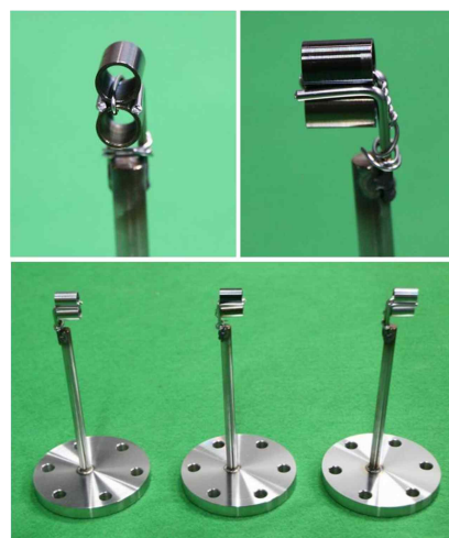
Fig. 2. Photograph of the corrosion specimen.
