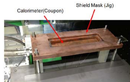
Fig. 2. Test mockup for the thermo-hydraulic calorimetry.
