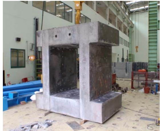
Fig. 2. SC Wall specimen
