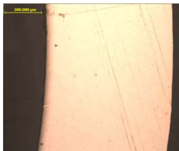
Fig. 1. SEM of cross-sections after 1500h at 470 °C.
