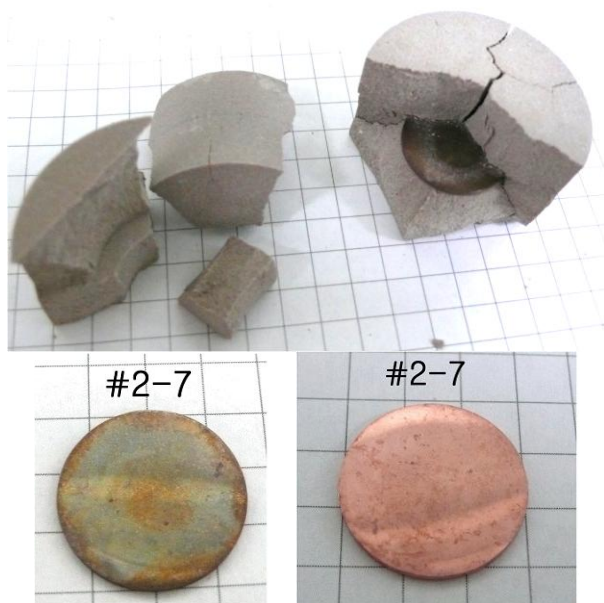
Figure 2. Copper specimen after a 9 month corrosion test.
