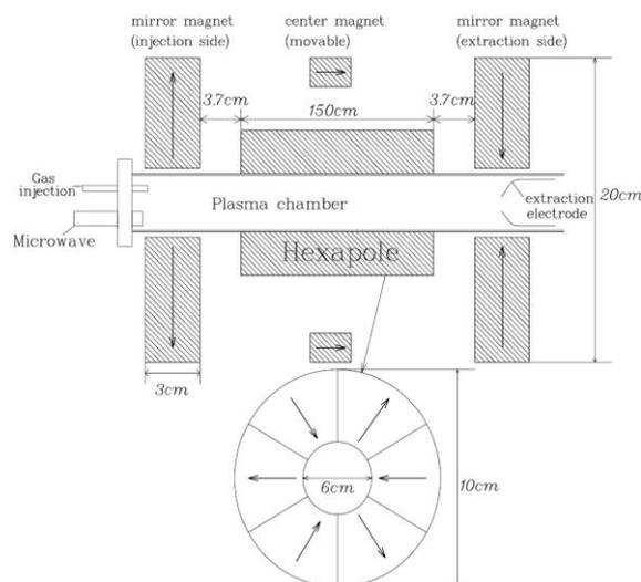
Fig. 1. Schematic view of Prototype of ECRIS at 2.45 GHz
