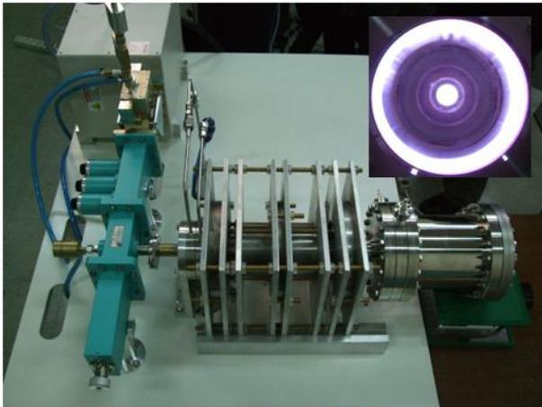
Fig.3. The figure shows 2.45GHz ECR ion source and small figure shows test result of plasma ignition.
