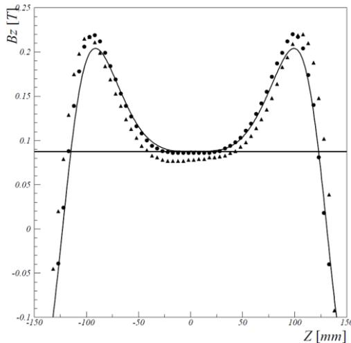
Fig.2. The measured field distribution (triangles) is compared with the OPERA-3D simulation result (solid line). Closed circles indicate the magnetic field distribution measured with a shorter distance between solenoid mirror magnets, which fits more with the simulation result.
