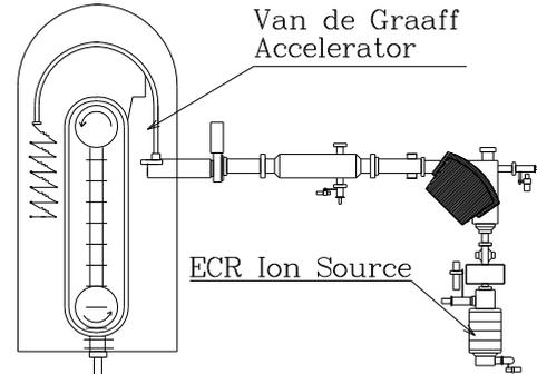
Fig.4. Schematic view of radioactive ion beam line with KBSI-ECR ion source and Van de Graaff Accelerator.
