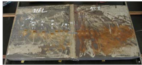
Fig. 1 Butt welded plate of stainless steel type 316L and SA508 steel.
