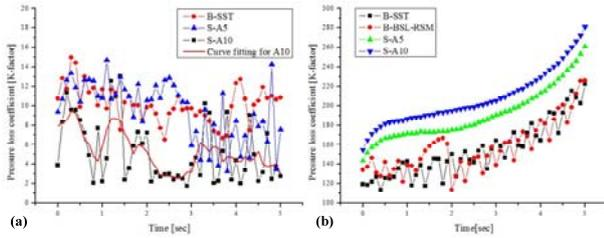
Fig.1. Pressure loss coefficient of the FD in the B and S-A Analysis: (a) high flow mode and (b) low flow mode
