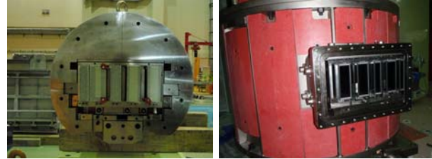
Fig. 5. Assembling guide cassettes into the in-pile plug and the primary shutter
