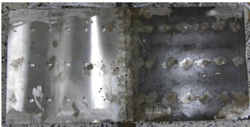
Fig. 1 Butt weld specimen
