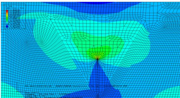
Fig. 6 Deformation of the CMD and the stress distribution (S11) of the 3<sup>rd</sup> overlay weld
