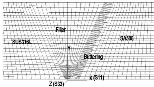
Fig. 2 2D FEM model of Butt weld
