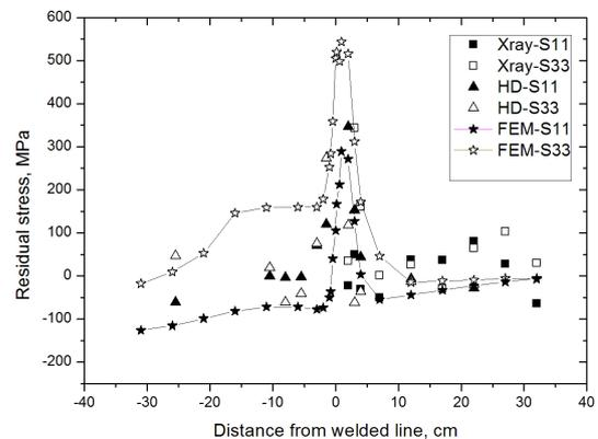
Fig. 3 FEM results of Butt weld
