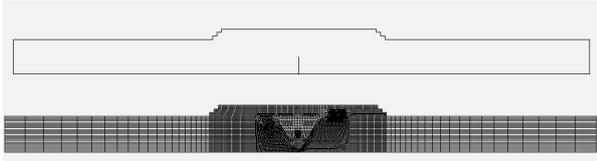
Fig. 4 2D FEM model of the Overlay weld
