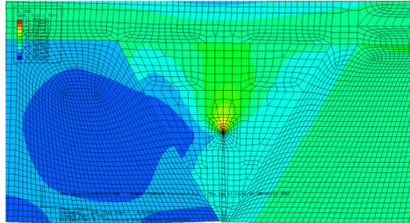
Fig. 7 Deformation of the CMD and the stress distribution (S33) of the 3<sup>rd</sup> overlay weld
