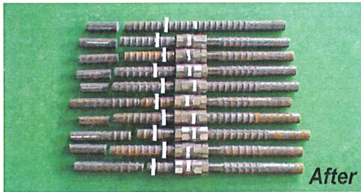
Fig. 4. Shapes of #18 rebar's failure
