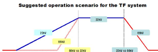
Fig. 1. Suggested operation scenario for the ITER TF coil AC//DC converter to decrease the DC short current.
