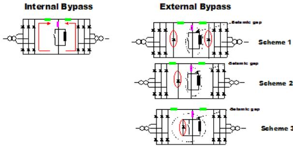
Fig. 2. Possible bypass methods of the ITER coil current.
