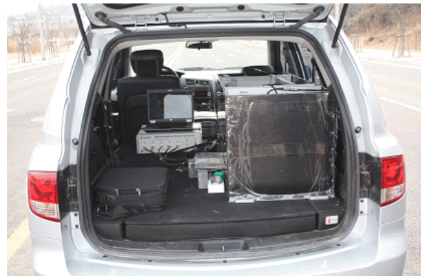
Fig. 2. The radiation system installed in a mobile unit
