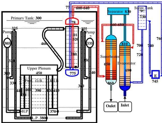
Fig. 3 MARS-LMR Nodalization for EBR-II plant
