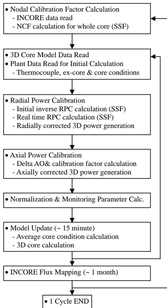
Figure 1. Online Core Monitoring Program Flow Chart
