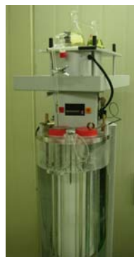
Fig.1. A density gradient column to measure the density of SiC coating layer of coated particles.
