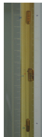
Fig.3. A gradient density solution for density measurement of SiC coating layer of coated particles.
