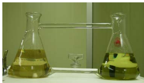
Fig.2. A flask with the lower density solution in the left side and a flask with the higher density liquid in the right side to make a density gradient solution.
