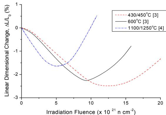
Fig. 1 Dimensional change with fast neutron dose
