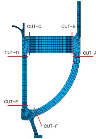
Fig. 5 Finite element model and cut locations for fatigue analysis
