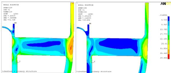
Fig. 3 Stress intensity distributions (left: maximum differential pressure, right: minimum differential pressure)
