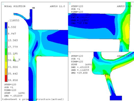
Fig. 4 Stress intensity distributions (actual differential pressure)
