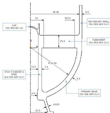
Fig. 1 Geometry of the tubesheet/shell juncture
