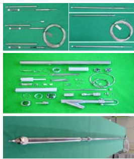
Figure 1. Instrumented capsule for nuclear fuel
