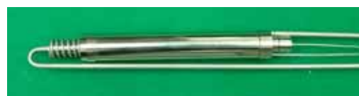
Fig. 4. A Double Cladding Fuel Rod (before and after assembling)
